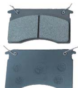
HBCG-PADS Brake Caliper Pads (Pair) To suit HBCG-L / HBCG-R
