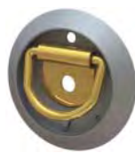
LR50ZP Lashing Ring Recessed SWL 250kg This useful steel tie-down is supplied complete with moulded shroud for plant-on fixing to wall or floor.
